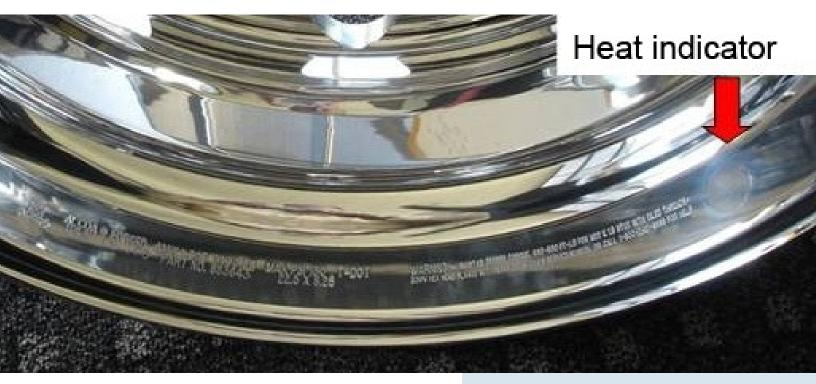
As tyres age, the heat generated from road friction causes tyres to become brittle. Rubber can crack, split or leak regardless of how much tread is on the tyre. When it comes to the wheel, significant events such as excessive heat from fire, brake malfunction, wheel bearing failure and other sources can weaken the metal, causing the tyre/wheel assembly to explode. Therefore, it is important to schedule wheel maintenance checks regularly.
